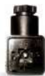
1578501 Quick connection connector DIN 43650, suitable for all IM2 coils. Cable gland Pg9 (cable diameter 6÷8 mm). Pg11 cable gland thread; Adjustable cable outlet in 4 positions every 90°.
