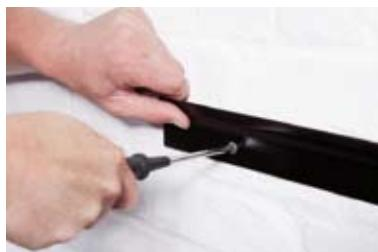
The hanging system is integrated in the back of the fireplace. First mount the top wall bracket, using good quality plugs and screws that suits your type of wall, then lift the fireplace up ensuring that the rear ledge of the fireplace engages the top wall bracket and is sitting centrally positioned on the bracket.
